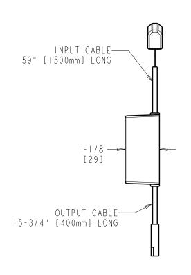
DIMENSIONS ARE IN INCHES AND [MILLIMETERS].
