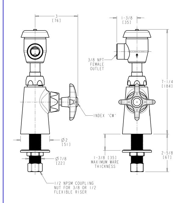
DIMENSIONS ARE IN INCHES AND [MILLIMETERS].
