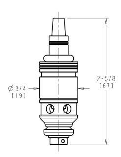
DIMENSIONS ARE IN INCHES AND [MILLIMETERS].
