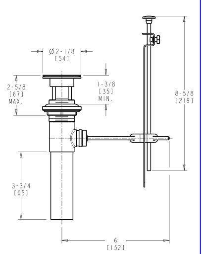
DIMENSIONS ARE IN INCHES AND [MILLIMETERS].
