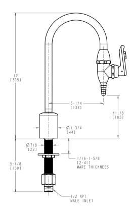
NOTE: HIGH PURITY PLASTIC VALVE IS NOT A CHEMICALLY INERT MATERIAL AND SHOULD NOT BE WASHED WITH STRONG ACIDS.
