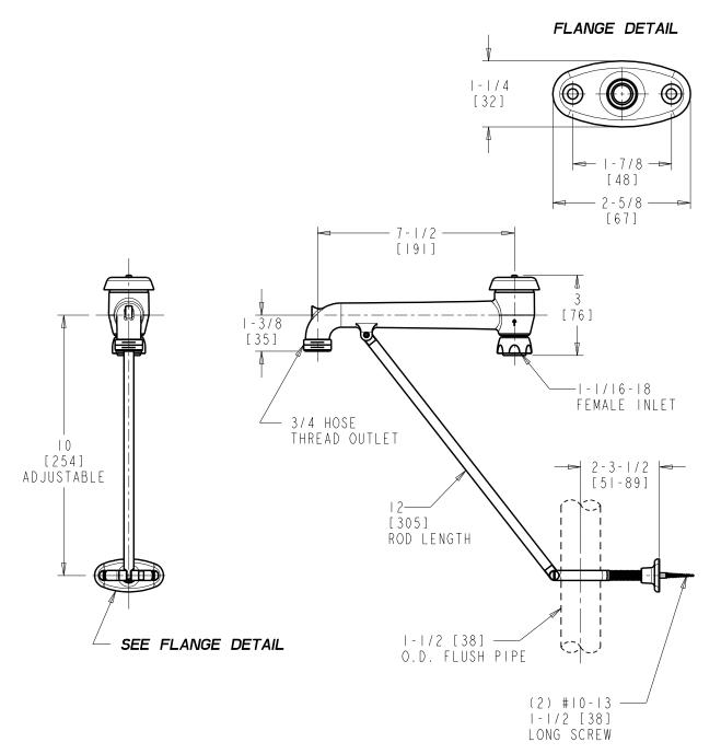
DIMENSIONS ARE IN INCHES AND [MILLIMETERS].
