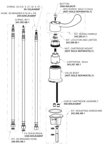
Cover Plate for Mechanical Mixing Valve with User Temperature Control **243.283.21.1**
