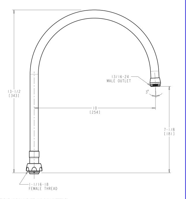
DIMENSIONS ARE IN INCHES AND [MILLIMETERS].
