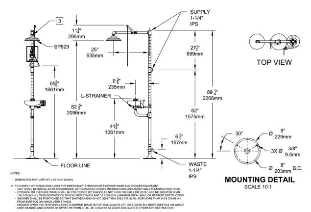
3. DO NOT USE REGULAR PIPE SEALANT. IF NECESSARY USE DOW CORNING 832 SEALANT PLACING 5 SMALL BEADS ON THE MALE THREADS, JUST ABOVE THE FIRST THREAD.
